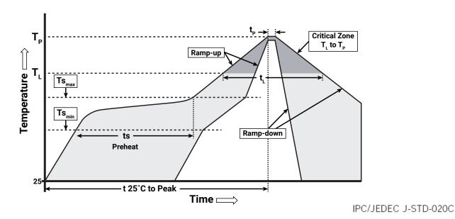
Profile FeatureLead-Free SolderTemperature Min. (Tsmin)150 °CTemperature Max. (Tsmax)200 °CTime (ts) from Tsmin to Tsmax60-120 secondsRamp-Up Rate (Tto Tp)3 °C/second
