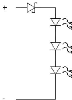
Figure 10: Schottky barrier diode in LED circuit
