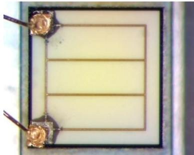
Figure 4: LED chip with damaged bond pads
