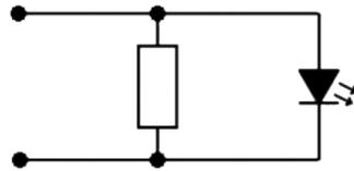
Figure 5: Overvoltage protection in parallel with LED
