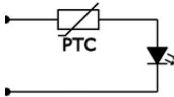
Figure 8: PTC resistor in series with LED
